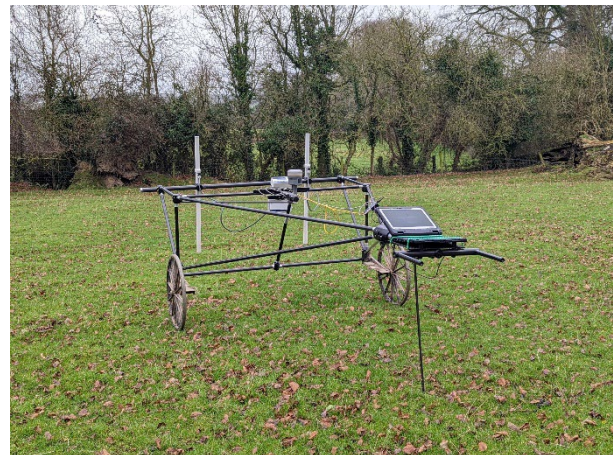
Bartington Grad 601-2 mounted on Bartington Cart
