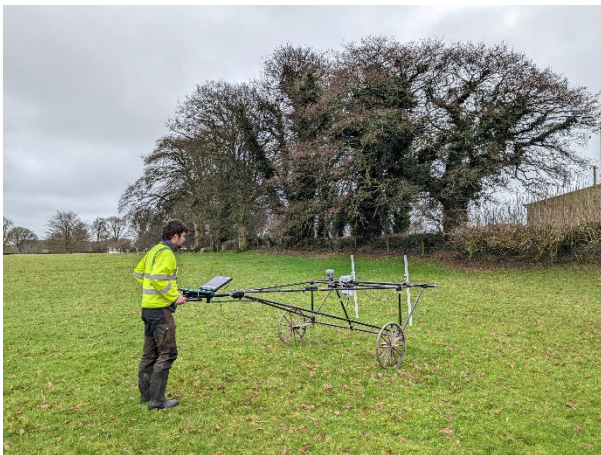
Bartington Grad 601-2 mounted on Bartington Cart
